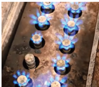
Gas Nozzle before Cleaning
