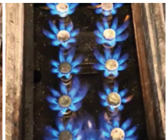
Gas Nozzle after Cleaning
